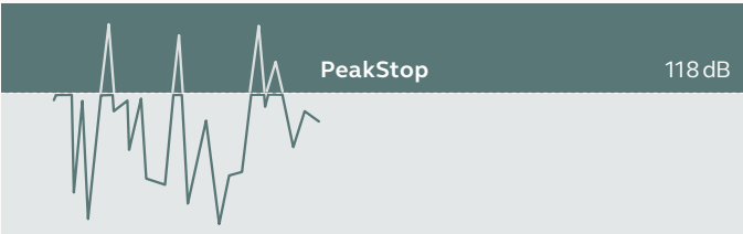
Fig. 2: PeakStop continuously monitors the sound flow and actively reduces critical sound peaks to a safe level.
